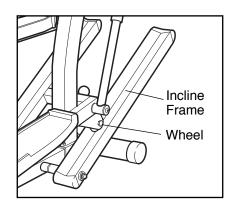
from the incline frame where the wheels make contact with it. Other parts of the elliptical crosstrainer can also be cleaned in this manner. **Never use abrasives or solvents.**
